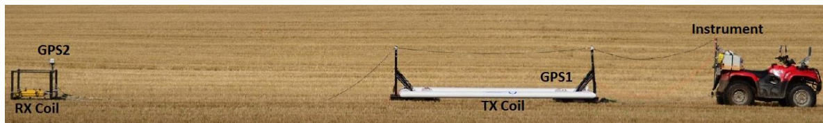
Figure 2. The tTEM system. For a detailed instrument setup see Error! Reference source not found.
